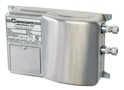
Instantaneous point of use water heater ideal for use with eye wash fountains. Designed for non-continuous use it is perfect for installations where the unit will require warm water at short notice without the need to store warm water for long periods of time. Stainless steel casing with Celcon waterways and Ni Chrome heating coils.
